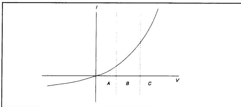
The curve indicates that for low microwave input levels (Region A), the single-diode detector output is proportional to the square of the input power. For high input signal levels (Region C), the output is linearly proportional to the input. In between these ranges (Region B), the detector response lies between square-law and linear.
