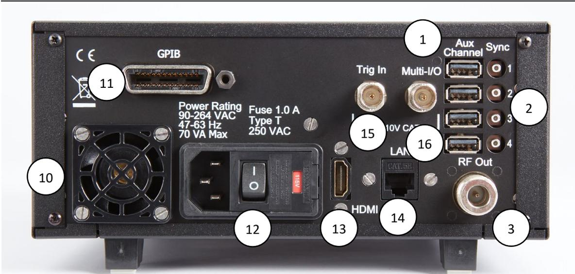
Figure 3-2. PMX40 RF Power Meter - Rear Panel
