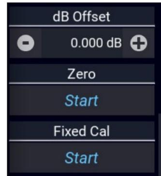
**Zero:** Performs a zero offset null adjustment. The sensor does not need to be connected to any calibrator for zeroing. This action removes the effect of small, residual power offsets, and should be performed prior to low-level measurements. The procedure is often performed in-system. There should be no RF signal applied to the sensor input prior to zeroing.
