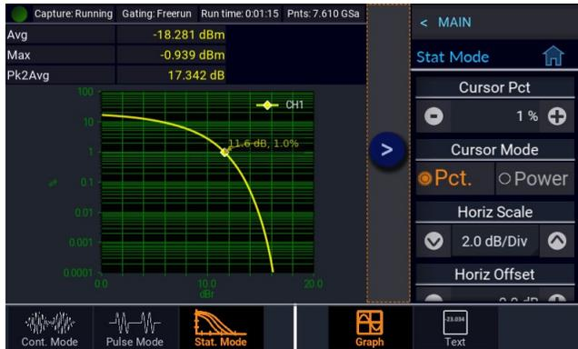
**Figure 3-8. CCDF Plot With Menu Showing Cursor at 1%**
