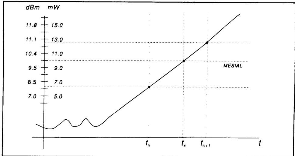
10. The process determines horizontal position, in pixels, at which the signal crosses the mesial value. This is done to a resolution of 0.1 pixel, or 1/5000 of the screen width. Ordinarily, the sample values do not fall precisely on the mesial line, and it is necessary to interpolate between the two nearest samples to determine where the mesial crossing occurred. This process is demonstrated in the example above (Figure 5-6):
