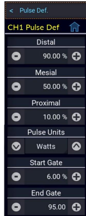
measurements between mesial crossings such as width and period are not affected. The purpose of the Pulse Gate setting is to exclude edge transition effects from the pulse power measurements.
