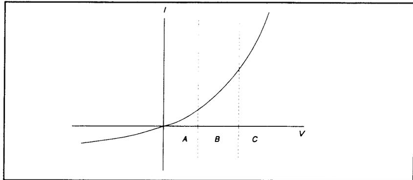
The curve indicates that for low microwave input levels (Region A), the single-diode detector output is proportional to the square of the input power. For high input signal levels (Region C), the output is linearly proportional to the input. In between these ranges (Region B), the detector response lies between square-law and linear.
