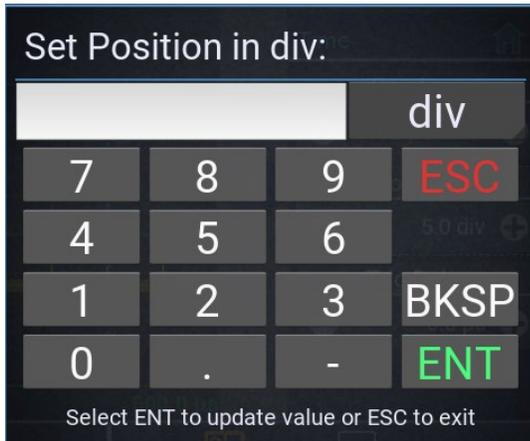
Figure 4-2. Channel 1 Vertical Center Numeric Keypad
