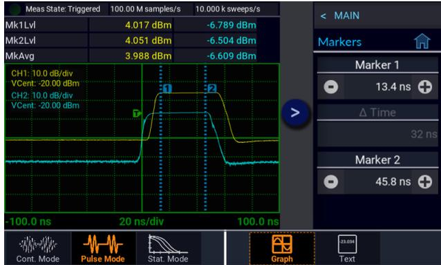
Figure 3-6. Marker Measurements on CH1 and CH2 Pulses
