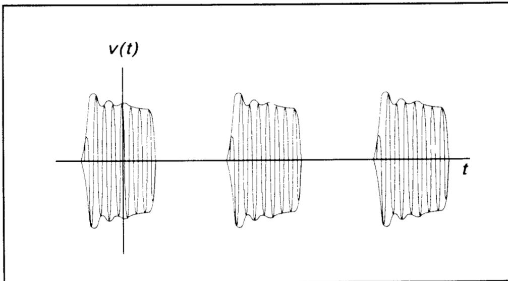
Figure 5-2. Distorted Pulsed Signal
