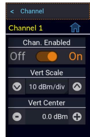
**Vert Center:** Set the power or voltage level of the horizontal centerline of the graph for the specified channel in the selected channel units.
