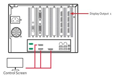
If a control screen is unavailable, connect a single video wall display into the Display Output 1 connector on the rear of the iolite 600.
