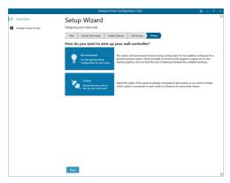
The DDCT can recommend the best wiring configuration for your system, ensuring the load is balanced between the graphics hardware. Click on **Recommended** for the optimal configuration for your system.
