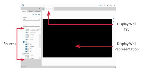
When opened, the display wall tab shows a live representation of the physical wall and the sources available to display on it. To place a source on the video wall, simply click on the required source in the Sources Tab and drag it onto a preferred position on the display wall representation.
