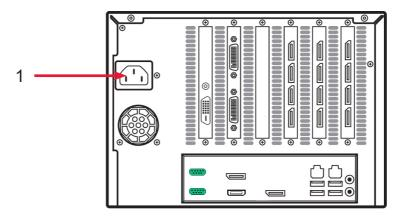
1 Connect power cables then plug into a mains supply.
