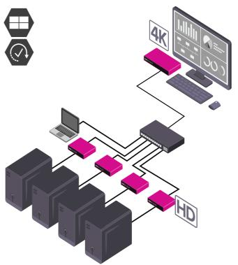
Window**View** allows space saving with easy monitoring and control. Manage up to four PC's from a single 4K monitor; while using only a single keyboard and mouse to control the PC of your choice. Going full screen is simple. One keystroke will make the source you are hovering over fill the 4K screen. If you want to go large, link up to sixteen sources across four displays.
