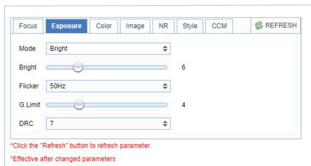
Figure 24: WebGUI > VIDEO > Camera Settings > Bright Exposure Mode
