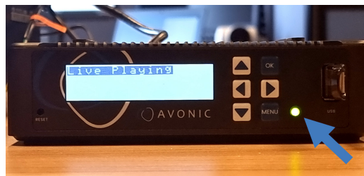
REC200 is live streaming video - > [OK] - > pause streaming
