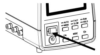
Insert the connector on the output side of the AC adapter to the DC input connector of the instrument.
