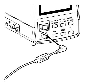
3 Plug in the AC adapter plug into the power outlet.
