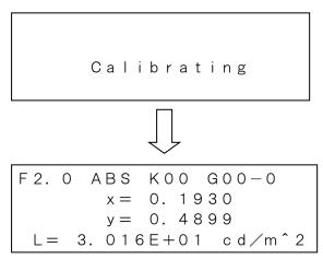
To finish measurement, press the RUN/HOLD switch. The final measurement results of continuous measurement will be displayed.
