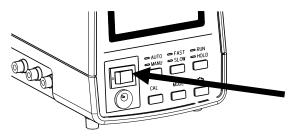
After the power has been turned ON, the instrument will warm up for 10 minutes, then the zero-adjustment starts and then measurement starts automatically.
