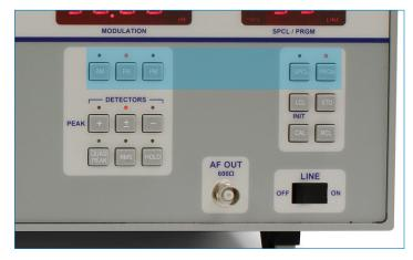
Figure-4: Function Keys of 8201A Modulation Analyzer
