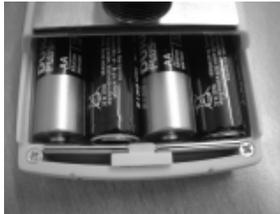
If the battery symbol appears in the measuring window resp. if a critical charge of battery is shown in the status, the batteries have to be changed IMMEDIATELY. If you do not use your moisture meter for a longer period, remove the batteries. For eventual resulting damages we cannot provide any warranty.
