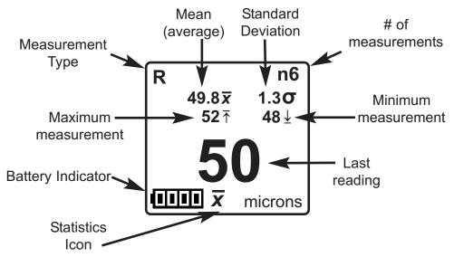
Remove the last measurement by pressing the (-) button. Press (+) to clear statistics.
