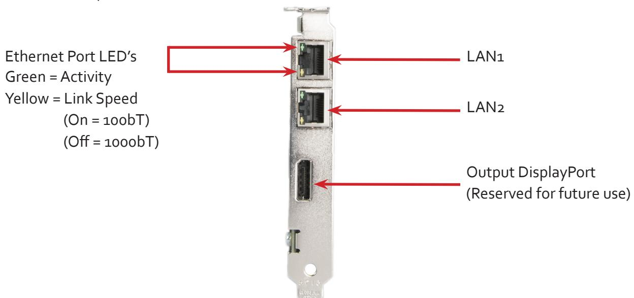
Connect a network cable into one or both of the Ethernet ports. Care should be taken when connecting a network cable, ensure the cable connector is pushed firmly into the Ethernet port until you hear a definite click. Failure to connect the network cable properly could result in the network connection being lost.
