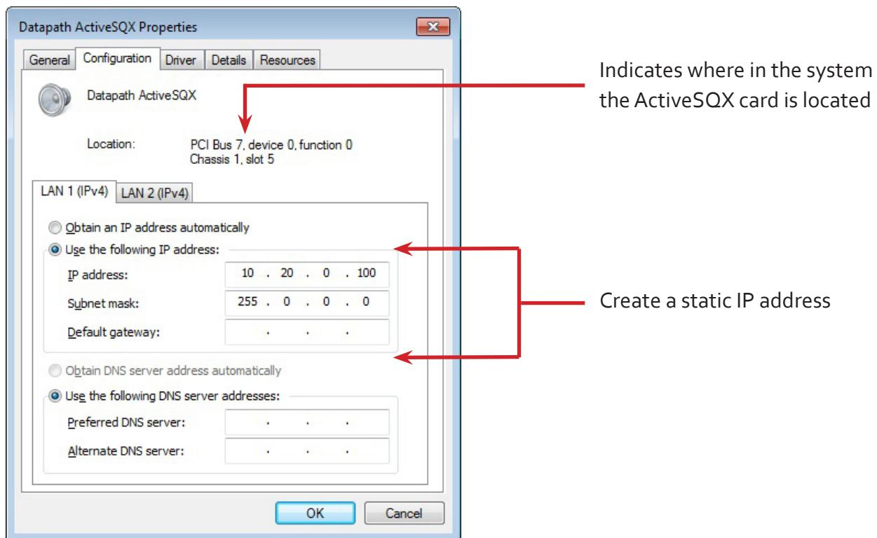
LAN1 and LAN2 operate independently therefore, should both require configuring as a Static IP address then this process should be repeated for LAN2 by clicking on the LAN2 tab.
