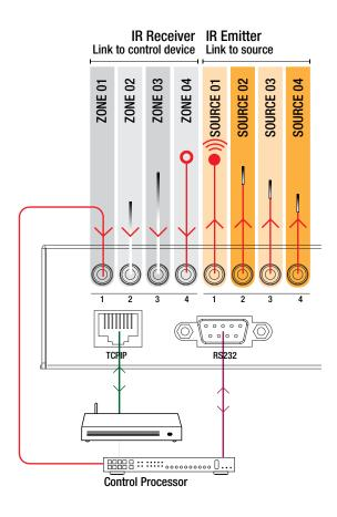
The Seamless HDMI Matrix is easily configured and added to ELAN projects using ELAN's Configuration Software. The EL-4KM-VW44 also features a web browser interface module for control and configuration of the matrix when used stand-alone or with a third party control system. Control options include front-panel push buttons, IR remote control, RS-232 interface, and TCP/IP.
