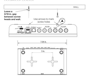
Structured Wiring Cabinet Mounting: The EL-IPD-PRE-SIO can be mounted using the optional Structured Wiring Cabinet Mount (EL-SC-100-BKT).
