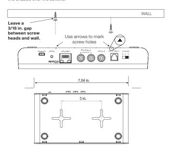
Structured Wiring Cabinet Mounting: The EL-IPD-PRE-SSI can be mounted using the optional Structured Wiring Cabinet Mount (EL-SC-100-BKT).
