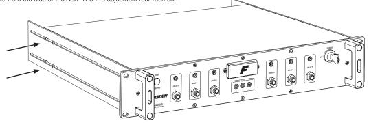
2. Reverse the rack ears and reattach the rack ears to the chassis (as shown here).
