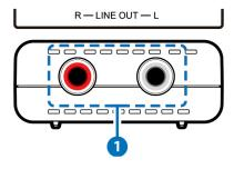
1 R/L LINE OUT: Connect the R/L analog audio output to the input of your Amplifier or audio system.
