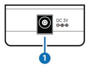
1 DC 5V: Connect the 5V DC power supply to the unit and plug the adaptor to an AC outlet.
