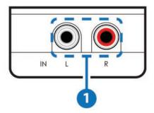
1 L/R IN: Connect to the source equipment such as a DVD/Blu-Ray player with stereo RCA cables to receive the audio signal.
