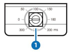
1 Lip SYNC Switch: This switch has eight settings that allow users to set the audio output delay from 0~300 milliseconds in order to perfectly synchronize audio and video signals.
