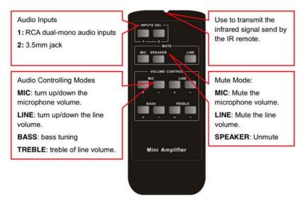
IR receiver head, works in conjunction with the IR remote. Please point the IR remote at the IR receiver when use, to avoid getting out of control as there is no signal detected.
