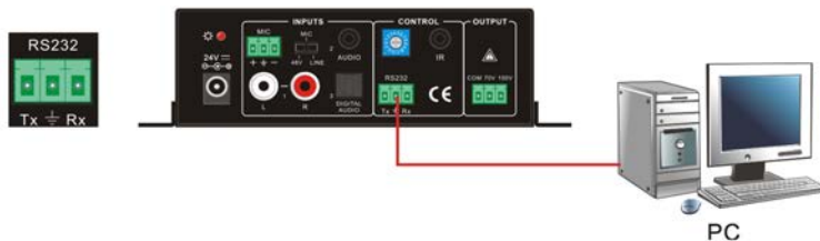
Figure 10 Connection of RS232 Port
