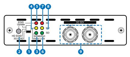
1 EDID Switch: Use this switch to select between the built-in or to update the EDID settings. Default EDID settings as shown below:
