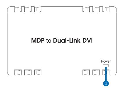
1 Power LED: When the USB cable is connected with power supply this power LED will illuminate in red.
