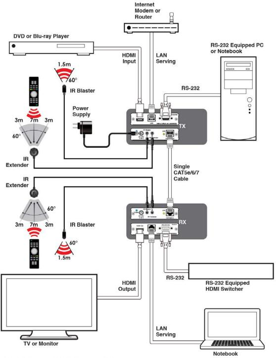
Note: Only a single unit needs to be powered and can power the other unit via PoC. In this example the Transmitter powers the Receiver.
