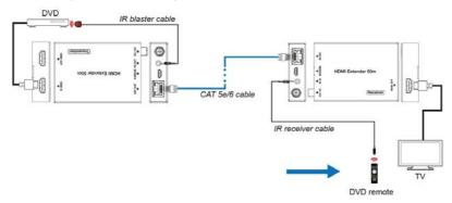
Note: IR remote sends signal distance for 0~5 meters / 0~8 meters, and angle is plus-minus 45 degrees / vertical direction .
