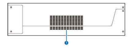
**FAN VENT:** These are air ventilation areas. DO NOT block these areas or cover them with any objects. Please allow adequate space around the unit for air circulation.
