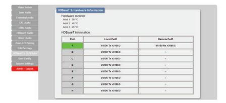
This page provides information concerning the temperature inside the matrix (areas 1, 2 & 3) and the HDBaseT firmware versions used in the matrix and in connected receivers. Temperature area 1 is the left side of the output ports (from the front), area 2 is the right side of the output ports (from the front) and area 3 is at the middle of the HDMI inputs.
