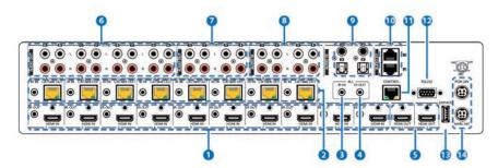
**HDMI IN & IR OUT 1~10:** Connect up to 6 source devices to the HDMI ports using appropriate quality HDMI cables. Input source devices include Blu-ray players, set-top boxes, game systems and so on. These inputs are DVI-D compliant (with the use of DVI to HDMI adapters or cables). Attach IR blasters to the IR Out ports to transmit the IR signals received from connected HDBaseT Receivers. The IR signal routing follows the HDMI signal routing.
