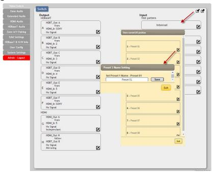
This matrix can store up to eight video and audio routing presets. Presets can be utilized to store multiple different routing states in advance for rapid, hassle-free, recall.
