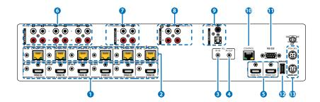
**1 HDMI IN & IR OUT 1~6:** Connect up to 6 source devices to the HDMI ports using appropriate quality HDMI cables. Input source devices include Blu-ray players, set-top boxes, game systems and so on. These inputs are DVI-D compliant (with the use of DVI to HDMI adapters or cables). Attach IR blasters to the IR Out ports to transmit the IR signals received from connected HDBaseT Receivers. The IR signal routing follows the HDMI signal routing.
