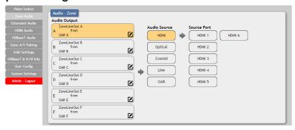
Click the buttons from left to right to choose each output's source. Once the new source has been selected, the change will happen immediately. Audio source options include HDMI, Optical, Coaxial, Line, and OAR.
