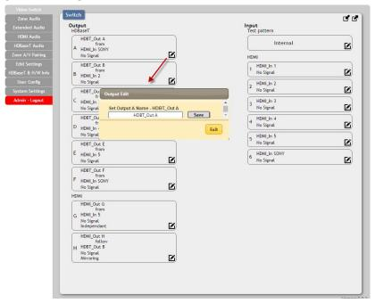
All inputs and outputs can be renamed as required. To rename the HDBaseT output ports and HDMI input ports please click the "edit" icon (②). Click the "Save" button to confirm the change.
