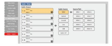
Click the buttons from left to right to choose each mixer's A & B sources. Only 2 sources total may be selected for each mixer. Once the new source has been selected, the change will happen immediately. Audio source options include HDMI, Optical, Coaxial, Line, OAR and Audio CAT.
