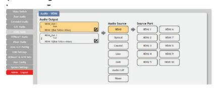
Click the buttons from left to right to choose each output's source. Once the new source has been selected, the change will happen immediately. Audio source options include HDMI, Optical, Coaxial, Line, OAR, Audio CAT and Mixer.
