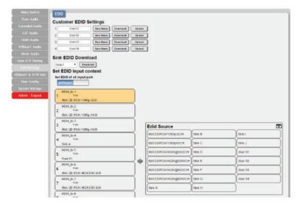
The Set EDID Input Content section allows for the assignment of an EDID to each individual input port, or to all inputs at once. Click the selection bar to toggle between individual assignment, or all inputs.
