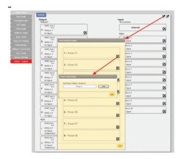
This matrix can store up to eight video and audio routing presets. Presets can be utilized to store multiple different routing states in advance for rapid, hassle-free, recall.
