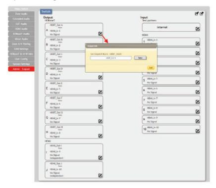
All inputs and outputs can be renamed as required. To rename the HDBaseT output ports and HDMI input ports please click the "edit" icon ( **②** ). Click the "Save" button to confirm the change.
