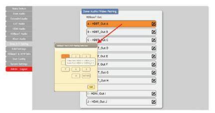
Please select the HDBaseT output port first and then click the "edit" icon ( ☑ ) to launch the window for further adjustments. The numbers 1~10 and "pattern" correspond to the keys on remote control unit.
