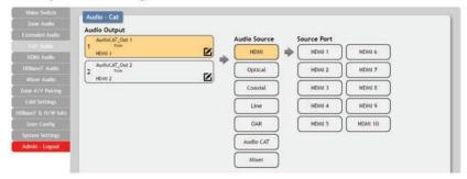
Click the buttons from left to right to choose each output's source. Once the new source has been selected, the change will happen immediately. Audio source options include HDMI, Optical, Coaxial, Line, OAR, Audio CAT and Mixer.
