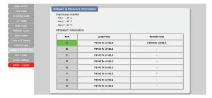
This page provides information concerning the temperature inside the matrix (areas 1, 2 & 3) and the HDBaseT firmware versions used in the matrix and in connected receivers. Temperature area 1 is the left side of the output ports (from the front), area 2 is the right side of the output ports (from the front) and area 3 is at the middle of the HDMI inputs.
