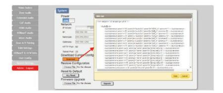
Click the "Download" button to save the current system configuration to your local PC. The current system configuration will be saved as XML file. The system configuration can also be restored from a saved XML file by clicking the "Choose File" button to locate the saved XML file, then clicking the "Restore" button.
