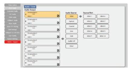
Click the buttons from left to right to choose each output's source. Once the new source has been selected, the change will happen immediately. Audio source options include HDMI, Optical, Coaxial, Line, OAR, Audio CAT and Mixer.
