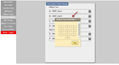
Please select the HDBaseT output port first and then click the "edit" icon (☑) to launch the window for further adjustments. The numbers 1~10 correspond to the keys on remote control unit.
