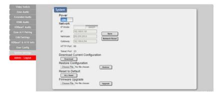
This page provides system configuration options including turning the power on/off, changing the network settings, downloading/restoring saved system configurations, resetting the system to factory defaults and updating the firmware.
