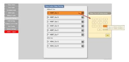
Please select the HDBaseT output port first and then click the "edit" icon ( ☑) to launch the window for further adjustments. The numbers 1~10 and "pattern" correspond to the keys on remote control unit.
