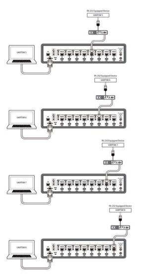
Note: This command allows RS-232 to control the RS-232 device connected to output E's Receiver.
