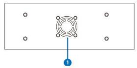
**Fan Ventilator:** These are air ventilation areas, DO NOT block these areas or cover it with any object. Please allow adequate space around the unit for air circulation.
