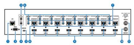
1 LAN: Connect to an active network for LAN serving and Telnet and Web GUI control (refer to Sections 6.8 and 6.9). When the Matrix or any compatible LAN equipped receivers are connected to a network, this allows the network access (including internet access if available) to be shared between the Matrix and all connected receivers. Connect any Ethernet equipped device e.g. a Smart TV or games console to the LAN port of a receiver for that device to share the network/internet access.
