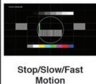
The **General** pattern is an all-purpose, multi-pattern test to visually check for multiple issues simultaneously. It includes color bars, 8-step greyscale, vertical and horizontal multi-burst, cross hatch, circle and motion patterns. There are 3 variations: No motion, slow motion and fast motion.
