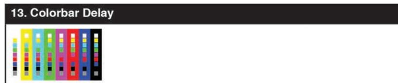
The **Colorbar Delay** pattern provides a sequence of standard 100% color bars with a full set of smaller color squares within each bar. This test is primarily to detect if any of the color components of the video signal are delayed/skewed relative to each other. Pay close attention to the left and right sides of the squares and look for a color shift. This is a common problem when using extreme-length analog extension products, or very long analog cables.
