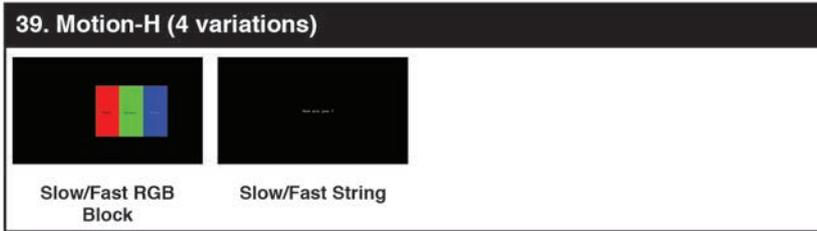
The **Motion-H** patterns are a collection of horizontal motion tests. These can be used to test your display’s pixel on/off response time. There are 4 variations: Slow red/green/blue block, fast red/green/block, slow moving sample text, fast moving sample text.
