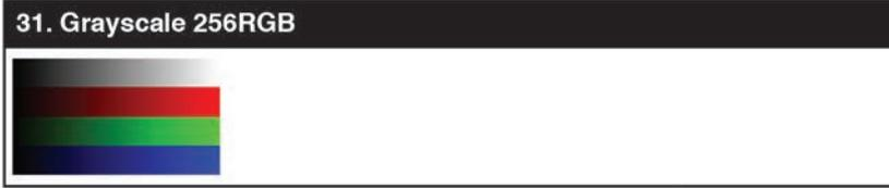
The **Grayscale 256RGB** pattern provides a way to fine tune the contrast, brightness, grayscale and color tracking of your display with a four full 265 step gradients (gray, red, green, blue) progressing from 0% to 100% brightness. When testing a display, the transition from dark to light should appear even and consistent across all 4 sections.
