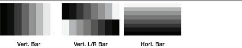
The **Grayscale 8** pattern provides a way to check and adjust the contrast, brightness and grayscale tracking of your display with 8 bars progressing from 0% to 100% brightness in even steps. When testing a display, no color should be visible in any of the bars, and all bars should be visible and distinct. There are 3 variations: 8 vertical bars, two sets of 8 vertical bars with the lower set reversed, and 8 horizontal bars.
