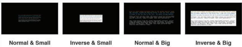
The **Text** pattern is used to check the clarity of text at various sizes and colors. This is primarily a test for projectors. There are 4 variations: Small multi-color text on a black background, small multi-color text on a white background, large multi-color text on a black background, and large multi-color text on a white background.
