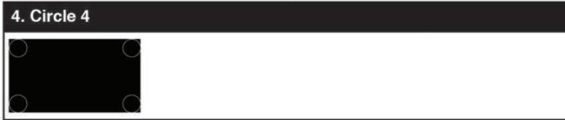
The **Circle 4** pattern provides 4 smaller white circles in each of the 4 corners of the screen. This pattern can help confirm that the display is maintaining correct geometry at the edges of the screen.
