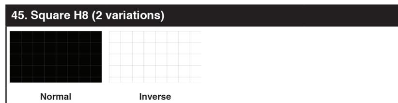
The **Square H8** pattern is a full field black & white pattern of squares dividing the screen horizontally into 8 sections. This pattern is primarily used to check projector linearity. There are 2 variations: Normal (white lines, black field) and Inverse (black lines, white field).
