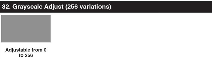
The **Grayscale Adjust** pattern provides a full field of grey with user adjustable brightness levels for testing display gray purity and signal response. The brightness can be freely adjusted from 0 to 255 by pressing the PATTERN button followed by the -/+ buttons. The gray level number will appear in text on screen while it is in adjusting mode.
