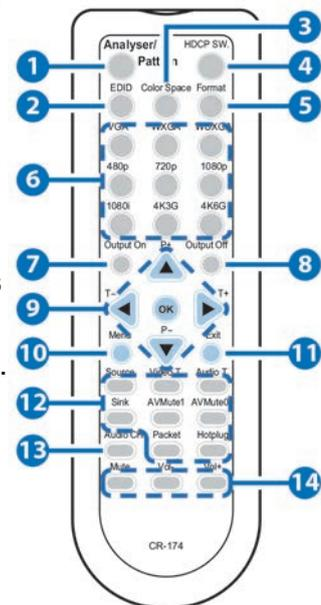
**P+/P-:** Press (+/-) to change the current test pattern. Within the OSD menu, press to move up and down.
