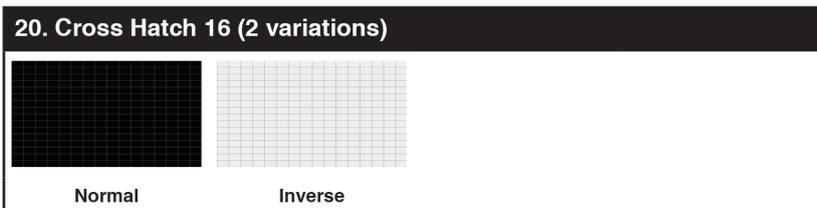
The **Cross Hatch 16** pattern is a full field black & white pattern of crossing vertical and horizontal lines dividing the screen into 16 sections in each direction. This pattern is primarily used to check for color convergence and pincushion issues in projectors. There are 2 variations: Normal (white lines, black field) and Inverse (black lines, white field).
