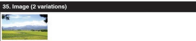
The **Image** pattern is a user customizable test pattern that holds two bitmap images. One image is for use with low output resolutions (below 1920x1080) and the other is for high output resolutions (1920x1080 and above). The low resolution image is a 640x480 bitmap (RGB, 24-bit) and the high resolution image is a 1920x1080 bitmap (RGB, 24-bit).
