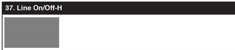
The **Line On/Off-H** pattern generates an alternating pattern of single-pixel horizontal white lines. This pattern can be used to analyze the vertical pixel resolution of your display. If the output appears to have mosaic patterns, or appears to be a solid gray field, then it is possible that your display does not fully support the resolution you are currently sending to it.
