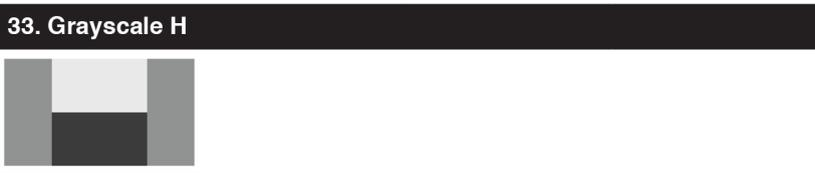
The **Grayscale H** pattern provides 4 distinct gray fields in an “H” arrangement for testing luminance transition stability. No color or interference should be visible at the transitions between sections.
