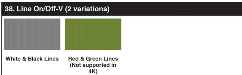
The **Line On/Off-V** pattern generates an alternating pattern of single-pixel vertical lines. This pattern can be used to analyze the horizontal pixel resolution of your display. If the output appears to have mosaic patterns, or appears to be a solid gray field, then it is possible that your display does not fully support the resolution you are currently sending to it. There are 2 variations: alternating white & black lines and alternating red and green lines.
