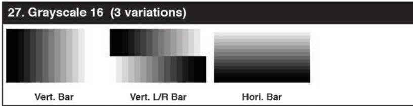
The **Grayscale 16** pattern provides a way to check and adjust the contrast, brightness and grayscale tracking of your display with 16 bars progressing from 0% to 100% brightness in even steps. When testing a display, no color should be visible in any of the bars, and all bars should be visible and distinct. There are 3 variations: 16 vertical bars, two sets of 16 vertical bars with the lower set reversed, and 16 horizontal bars.
