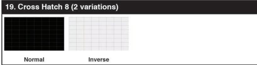
The **Cross Hatch 8** pattern is a full field black & white pattern of crossing vertical and horizontal lines dividing the screen into 8 sections in each direction. This pattern is primarily used to check for color convergence and pincushion issues in projectors. There are 2 variations: Normal (white lines, black field) and Inverse (black lines, white field).
