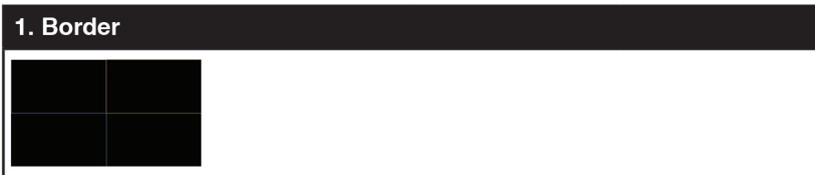
The **Border** pattern presents 4 equal-sized squares dividing the screen into 4 quadrants, forming a central white cross, with red, green, blue and white inner squares. Ideal for testing screen boundary, alignment and pincushion issues. All lines should be straight, and edge transitions should be sharp.
