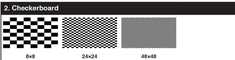
The **Checkerboard** pattern displays a repeating black and white checkerboard image. This is ideal for checking the alignment and corner convergence of TVs or monitors. Bandwidth can be checked by observing the vertical transitions. Transitions from black to white should be sharp. There are 3 variations: 8x8, 24x24 and 48x48.
