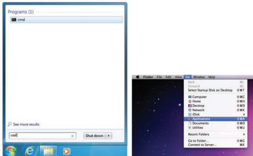
Once in the CLI (Command Line Interface) type “telnet” followed by the IP address of the unit and “23”, then hit “Enter”. The IP address can be found in the OSD within the “Ethernet” menu item.
