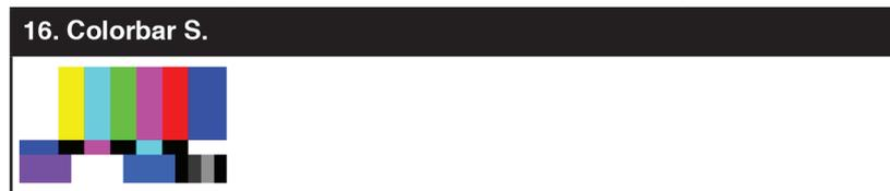
The **Colorbar S.** pattern is a standard SMPTE color bar pattern which is used for rapid verification of signal color accuracy and for display setup using the Blue-Only option on your display, if it has one.
