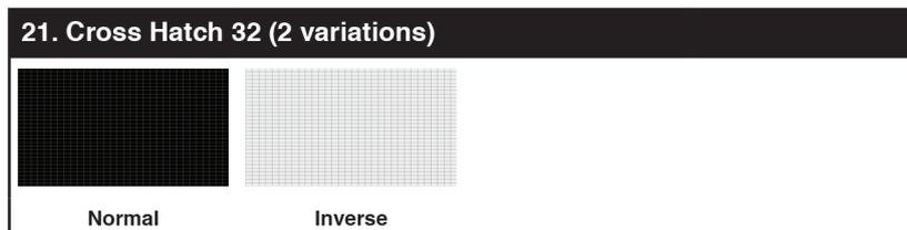
The **Cross Hatch 32** pattern is a full field black & white pattern of crossing vertical and horizontal lines dividing the screen into 32 sections in each direction. This pattern is primarily used to check for color convergence and pincushion issues in projectors. There are 2 variations: Normal (white lines, black field) and Inverse (black lines, white field).
