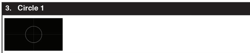
The **Circle 1** pattern provides a single white circle in the middle with a white cross and a white outer border line. This pattern is designed for quickly confirming that the geometry of the scene is correct and that the full source is being displayed, edge to edge.
