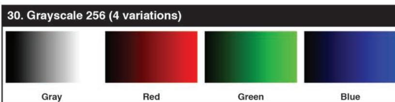
The **Grayscale 256** pattern provides a way to fine tune the contrast, brightness and grayscale tracking of your display with a full 265 step gradient progressing from 0% to 100% brightness. When testing a display, no color should be visible at any point across the gradient, and the transition from black to white should appear even and consistent. There are 3 variations: 256 vertical bars, two sets of 256 vertical bars with the lower set reversed, and 265 horizontal bars.
