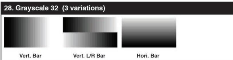
The **Grayscale 32** pattern provides a way to check and adjust the contrast, brightness and grayscale tracking of your display with 32 bars progressing from 0% to 100% brightness in even steps. When testing a display, no color should be visible in any of the bars, and all bars should be visible and distinct. There are 3 variations: 32 vertical bars, two sets of 32 vertical bars with the lower set reversed, and 32 horizontal bars.
