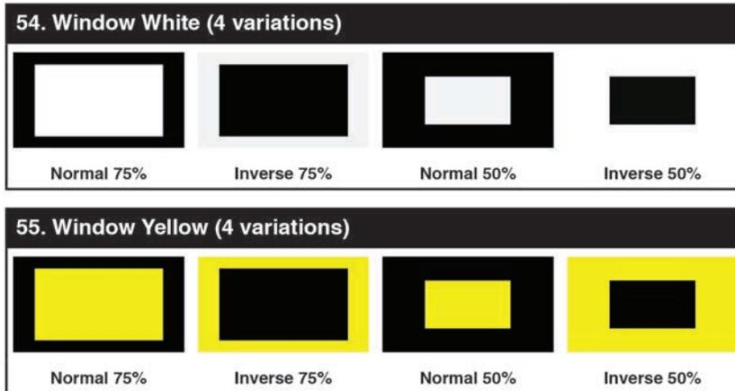
These **Window** patterns are additional screen purity tests offering seven different patterns with different sized windows of each color on a black field: **Blue, Cyan, Green, Magenta, Red, White, Yellow**. The color patterns should display an even distribution of brightness and consistent color tone across the screen. Each pattern has 4 variations: Normal 75% Window, Inverse 75% Window, Normal 50% Window, and Inverse 50% Window.
