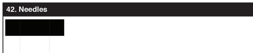
The **Needles** pattern is a standard needle pulse test. The top half of the screen is black and the bottom half is white with 2 thin inverse-brightness lines crossing from top to bottom. This pattern allows for analysis of the sharpness, blooming and screen distortion issues that a display might have.
