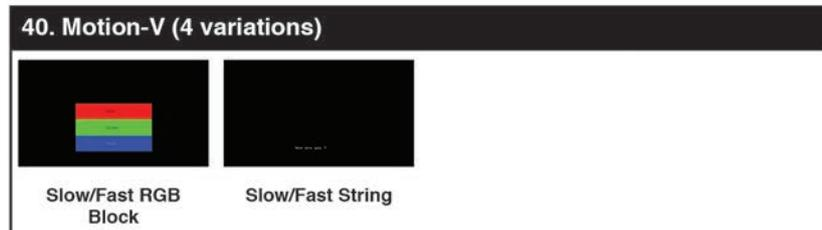
The **Motion-V** patterns are a collection of vertical motion tests. These can be used to test your display’s pixel on/off response time. There are 4 variations: Slow red/green/blue block, fast red/green/block, slow moving sample text, fast moving sample text.
