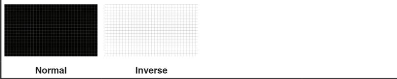
The **Square H32** pattern is a full field black & white pattern of squares dividing the screen horizontally into 32 sections. This pattern is primarily used to check projector linearity. There are 2 variations: Normal (white lines, black field) and Inverse (black lines, white field).
