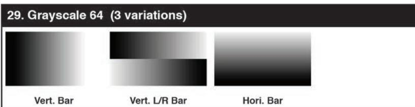
The **Grayscale 64** pattern provides a way to check and adjust the contrast, brightness and grayscale tracking of your display with 64 bars progressing from 0% to 100% brightness in even steps. When testing a display, no color should be visible in any of the bars, and all bars should be visible and distinct. There are 3 variations: 64 vertical bars, two sets of 64 vertical bars with the lower set reversed, and 64 horizontal bars.
