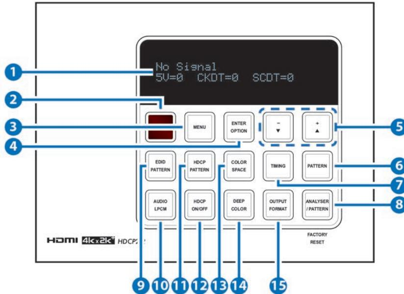
**1 OLED Screen:** Displays the current signal analysis information or test pattern mode selection details including input and/or output resolution timing. The screen layout changes completely depending on the unit's mode.
