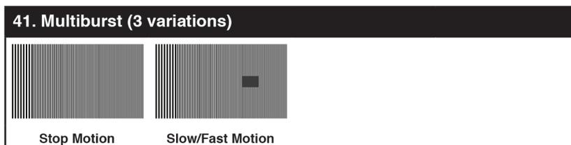
The **Multiburst** pattern provides a standard multiburst pattern consisting of vertical white lines that decrease in thickness from left to right allowing the user to analyze the bandwidth and frequency response of the video path and connected display. There are 3 variations: Standard multiburst, multiburst with a slow moving gray block, and multiburst with a fast moving gray block.
