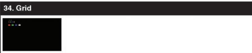
The **Grid** pattern provides a selection of red, green, blue and white boxes with 2x2 grids within and above them to test for pixel on pixel and color offset issues.
