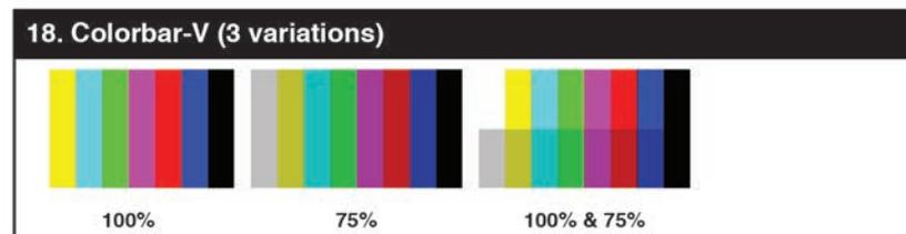
The **Colorbar-V** pattern comes in 3 variations. The first is a standard (white, yellow, cyan, green, magenta, red, blue, black) 100% color bar pattern using vertical bars. The 2nd variation has all bars at 75% brightness. The 3rd variation is split with the top half being at 100% and the lower half being at 75% brightness.
