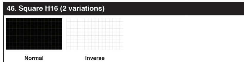
The **Square H16** pattern is a full field black & white pattern of squares dividing the screen horizontally into 16 sections. This pattern is primarily used to check projector linearity. There are 2 variations: Normal (white lines, black field) and Inverse (black lines, white field).
