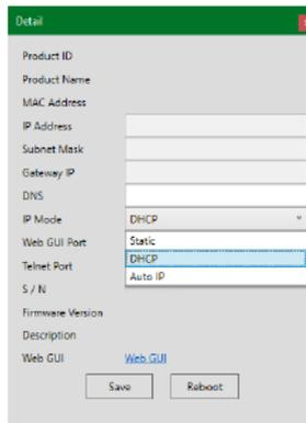
**1) IP Mode:** If you choose, you can alter the static IP network settings for the device, or switch the unit into DHCP mode to automatically obtain proper network settings from a local DHCP server. To switch to DHCP mode, please select DHCP from the IP mode drop-down, then click “Save” followed by “Reboot”.
