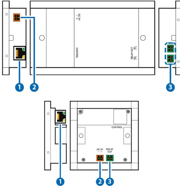
❶ CONTROL Port: Connect to an active Ethernet network via a switch or router to allow it to control other devices on the network and to be accessed via Telnet/WebGUI.
