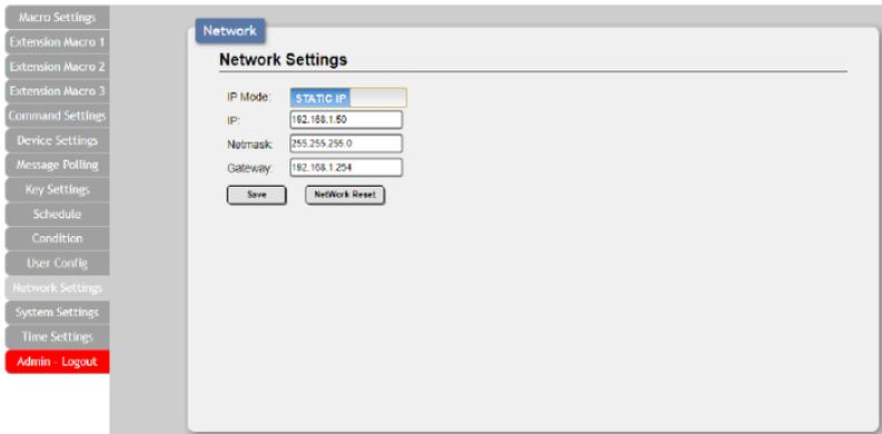
**1) Network Settings:** IP mode may be switched between Static IP or DHCP. In Static IP mode the IP, netmask and gateway addresses may be manually set. When in DHCP mode, the unit will attempt to connect to a local DHCP server and obtain IP, netmask and gateway addresses automatically. Please press “Save” after making any changes to the IP configuration or mode. To return all network settings to their defaults, press the “Network Reset” button.
