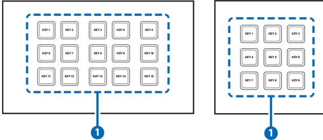
**1** KEY 1~15 (1~9) Buttons: Each button activates the customizable macro that has been assigned to it. All buttons contain a pair of colored LEDs (red and blue) with macro controllable individual brightness levels from 0~100.
