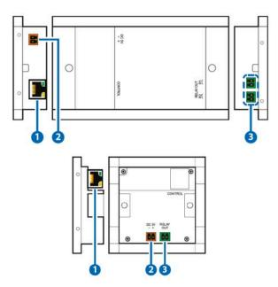
CONTROL Port: Connect to an active Ethernet network via a switch or router to allow it to control other devices on the network and to be accessed via Telnet/ WebGUI.
