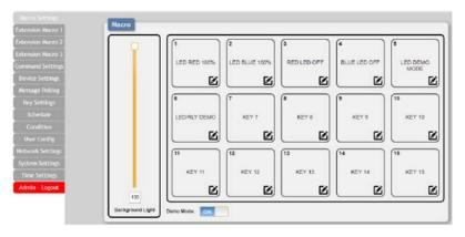
1) Macro Buttons: Press any of these buttons to activate the macro currently stored within it. Hovering the mouse over a button will list its current macro contents. Click on the edit *i* icon to edit each button's macro. There are 6 macros defined by default for testing the Wall Plate Control System's functionality. Click on macros 1~6 to demonstrate various LED light commands.
