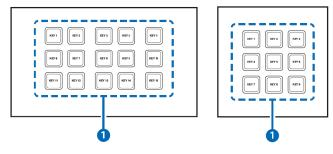
**1 KEY 1~15 (1~9) Buttons:** Each button activates the customizable macro that has been assigned to it. All buttons contain a pair of colored LEDs (red and blue) with macro controllable individual brightness levels from 0~100.
