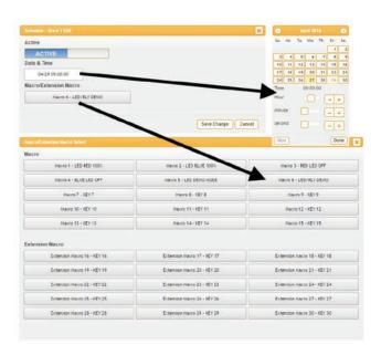
**Note:** This unit has 48 hours of backup power for the internal clock to protect against power loss and blackouts. After the backup power is exhausted the system time will reset back to 2015/01/01 00:00:00.
