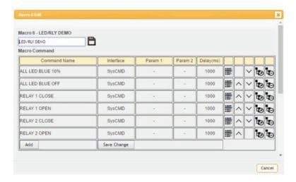
Click on the icon to insert a new command before the current one. Select one of the predefined commands from the list. (Details on how to create these pre-defined commands are later in this section.)
