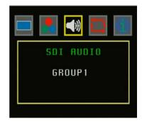
Selects the SDI audio output from 4 different audio groups and each group's 2CH contents or can be set to 'Auto' which contain up to 7.1 Channels of audio (dependent on the input source signal). If no audio output is required, the audio can also be muted by selecting 'OFF'.
