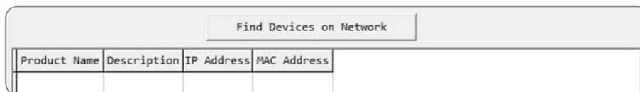
(3) By clicking on one of the listed devices you will be presented with the network details of that particular device. If you choose, you can alter the static IP network settings for the device, or switch the unit into DHCP mode to automatically obtain proper network settings from a local DHCP server. To switch to DHCP mode, please select DHCP from the IP mode drop-down, then click “Save” followed by “Reboot”.
