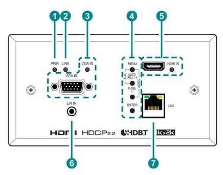
1 PWR LED: This LED will illuminate to indicate the unit is on and receiving power.
