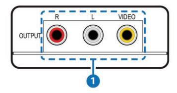
R/L/VIDEO OUTPUT: Connect to a TV/monitor and/or AV receiver with R/L & composite cable
