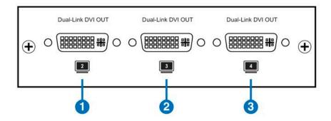
1 Dual-Link DVI OUT2~4: This slot is to connect with DVI output display with DVI cable for synchronize output with OUT 1.
