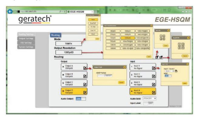
Click, drag, select or key-in on each selection setting to make the changes immediately. Click on the System setting for IP configuration setting. Both the device (from the OSD setting menu) and the web address entry bar will need to be reset once any change is made on this page.
