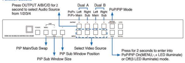
**Dual PiP mode:** To combine 2 sources to be presented on each HDMI output port (Dual A and Dual B) as main and sub screen image. The sub screen is in a part of the main screen.
