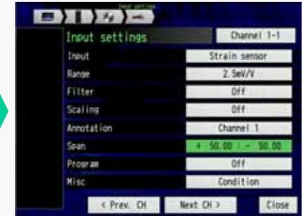
Select the "Span" for setting display signal range.
