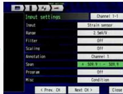
Select the "Span" for setting display signal range.
