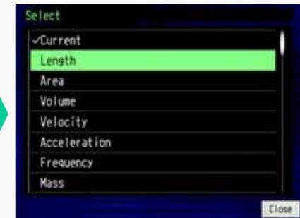
Select the type of signal for displaying the unit that has been pre-set.
