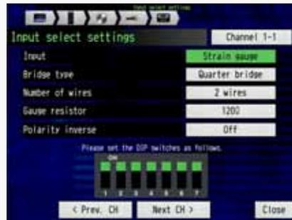
Set the "Input" to the "Strain gauge".
