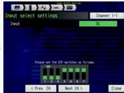
Set the Input to the "DC" for measuring the voltage.
