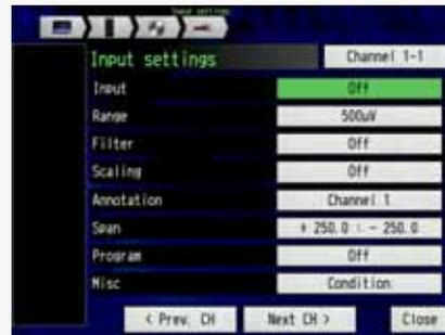
Select the "Input" for setting the type of input signal.
