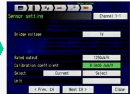
Settings of calibration coefficient (sensitivity of sensor) is displayed.
