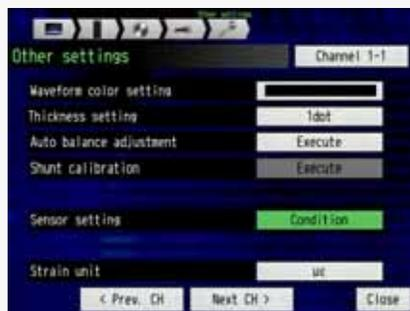
Select the "Sensor setting" for setting the condition of excitation for bridge circuit.
