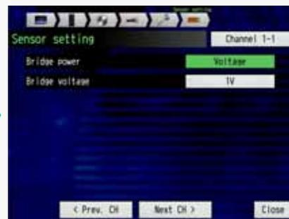
Select the "Bridge power" for setting the type of excitation for bridge circuit.
