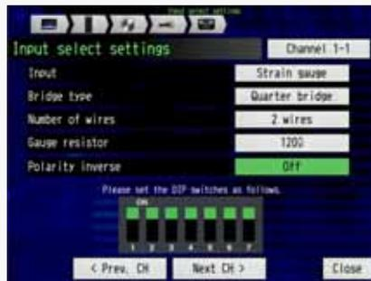
Select the "Polarity inverse" for setting polarity of signal.
