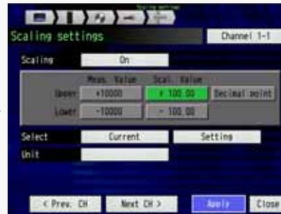
Select the "Upper" or "Lower" of the "Scal. Value". It will be the scaled value corresponding to the measurement value to column of the "Upper" and "Lower" of "Meas. Value".
