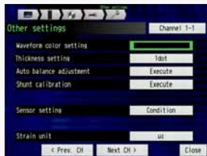
Press the "Execute" of the "Shunt calibration" for executing the shunt calibration.
