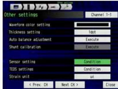
Select the "Sensor setting" for setting the sensor characteristics.
