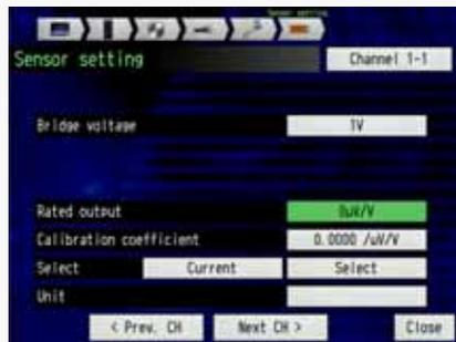
Select the "Rated output" for setting the sensor characteristic.
