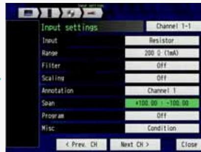
Select the "Span" for setting display signal range.
