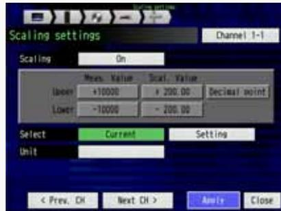
Select the "Select" for setting the type of scaled signal.
