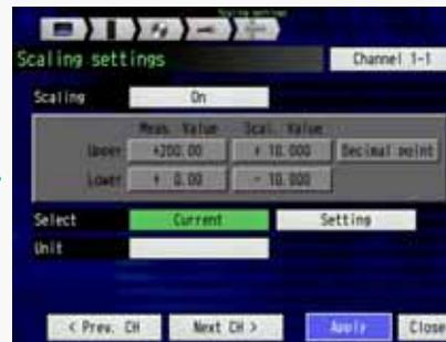
Select the "Select" for setting the type of scaled signal.
