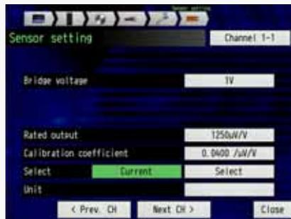
Select the "Select" for setting the type of measurement signal.
