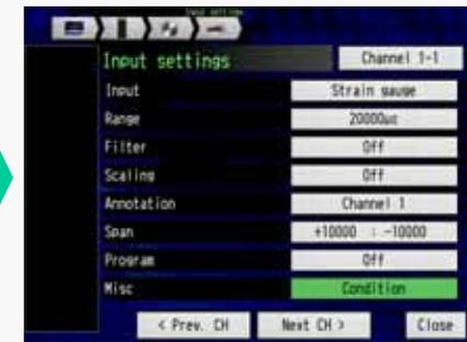
Select the "Misc" for setting the condition of bridge circuit.
