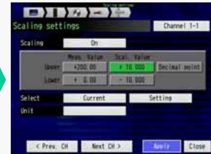
Select the "Upper" or "Lower" of the "Sal. Value". It is the scaled value corresponding to the measurement value to column of the "Upper" and "Lower" of "Meas. Value".
