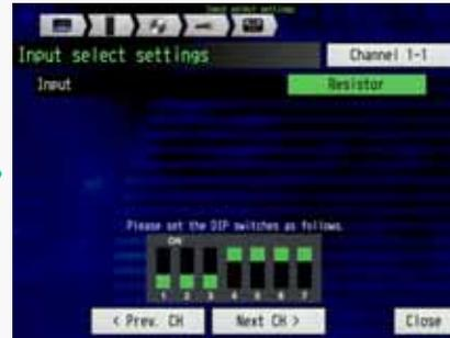
Set the Input to the "Resistor" for measuring the resistance.
