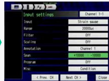
Select the "Span" for setting the displaying signal range.
