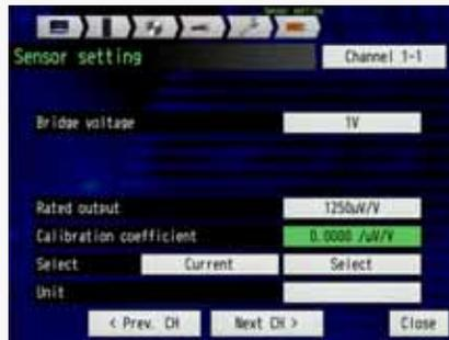
Select the "Calibration coefficient" for setting the sensor characteristics.
