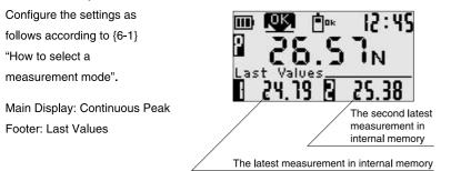
After the measurement exceed 10% of the gauge's capacity and fall to below 7% of the capacity, the peak value is transferred to Last Values.
