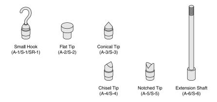
DSV(DST)-2N/5N/20N/50N come with aluminum attachments (A-type). DSV(DST)-200N/500N/1000N come with steel made attachments (S-type).
