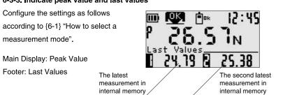
At the "Last Values", it indicates the measurement which is stored in internal memory\* by pressing SEND (SEND button). At [1], it indicates the latest value. At [2], it indicates the second latest value.
