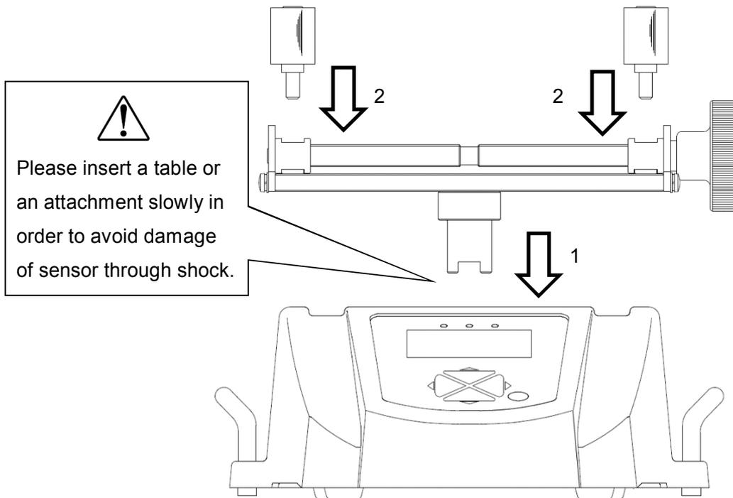
The torque sensor is at the inside of the mounting hole. Insert the shaft softly and horizontally and engage the sensor (1).
