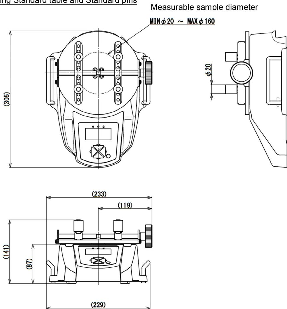
The no carry handle dimension for fixing the DTXS/DTXA with 4 holes.
