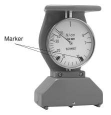
The instrument is equipped with two adjustable marks to mark a tension range which is mostly used.
