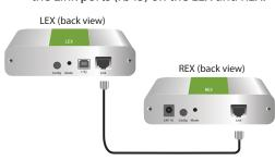
Connect the LEX to the computer using the included USB cable.
