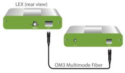
Max. distance between LEX and REX: Up to 50m with USB 3.0 storage type devices and up to 100m when using USB 3.0 bulk traffic cameras.
