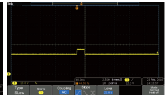
D/D Converter Surge Testing
