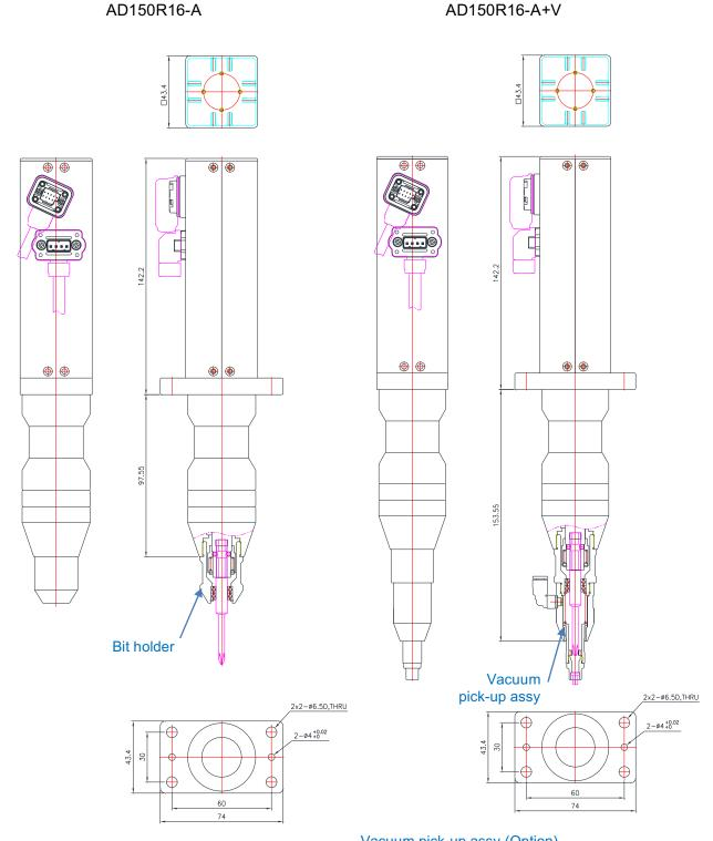
Bit holder (Option) for Ohmi V-17 or equivalent (Hex1/4" with Dia 7mm body hold by bearing )
