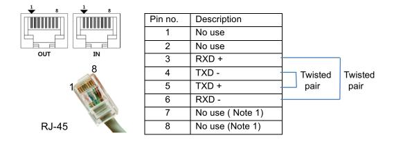
The pare of TXD+ / TXD- (4,5) and RXD+ / RXD- (3,6) wires should be twisted wiring.
