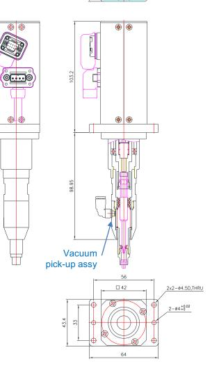
Bit holder (Option) for Ohmi V-17 or equivalent (Hex1/4" with Dia 7mm body hold by bearing)
