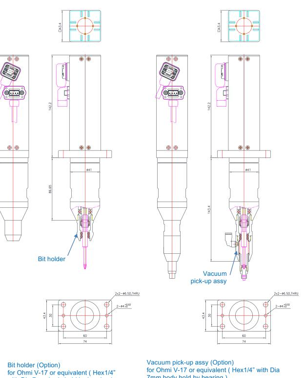
7mm body hold by bearing ) Mouth piece is not included in the assy. It is custom designed for each screw size and applications. The above described vacuum pick-up assy is for one of the application. It doesn't work for all application.
