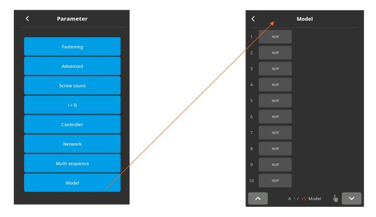
They are 15 sequencing models of 20 steps with assignable tightening program batch counting and logical IO management.
