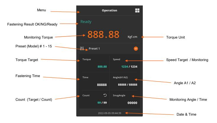
Operation screen is a default window when the controller power ON.
