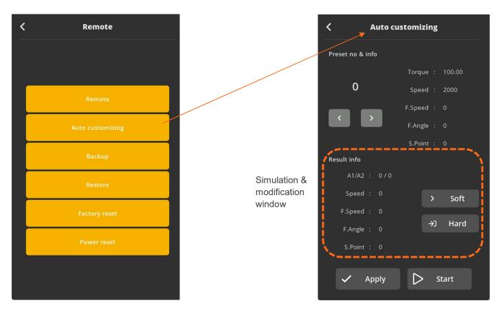
EC and ECT tool has the auto speed setting feature against torque setting to minimize over torque by speed shock. This auto speed is safe speed on the hard joint condition. On the real application, this setting can be changed manually. Auto customizing feature provides optimized parameter settings for saving cycle time on the real application.
