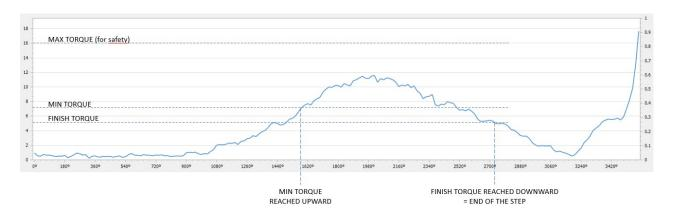
It is not the case in the chart (on prior page), but the tapping torque can be higher than the target torque (tapping in metal sheets, for example)
