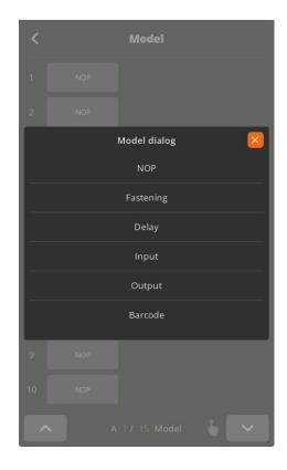
**Fastening setting**: The fastening with counting number follows all settings and features in Screw Count menu except the number of screw.
