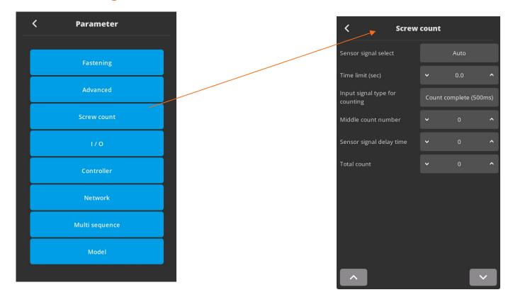
Screw count parameters are set for presets and models.
