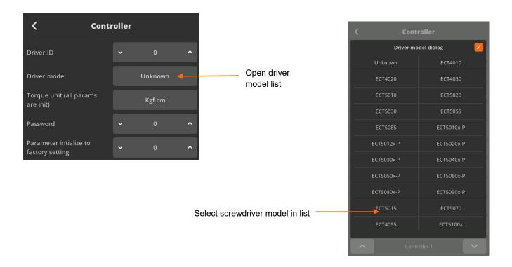
Power reset is done automatically and controller is initialized with selected screwdriver factory parameters.
