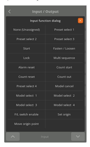
F/L switch enable: Allow reverse by external input when F/L switch is locked by controller setting
