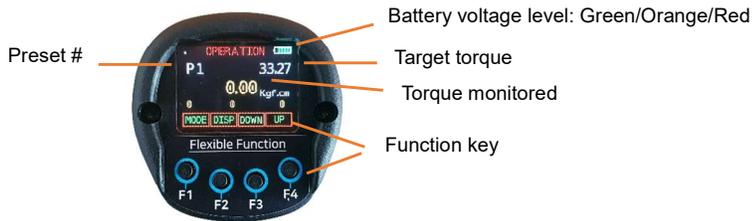
The operation mode screen is a default window when the screwdriver battery power is connected.
