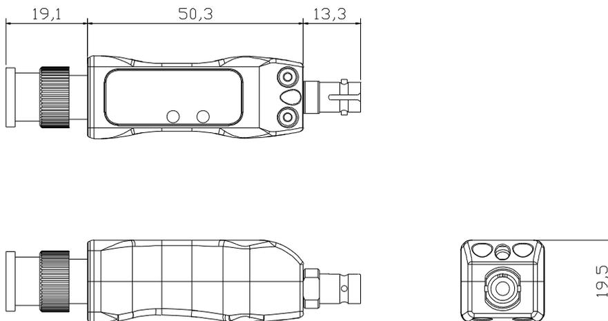
Note: The transmitter, SDISE-100-T and the receiver, SDISE-100-R have the same mechanical dimensions.
