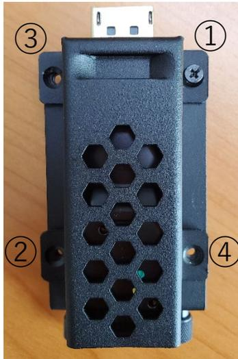
**Fig. 4: Holes to insert the screws**
