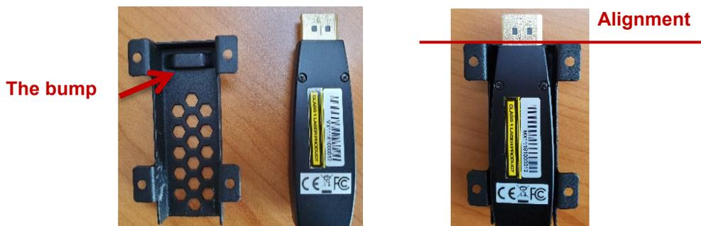
**Fig. 2: Insert the push button into the bracket**
