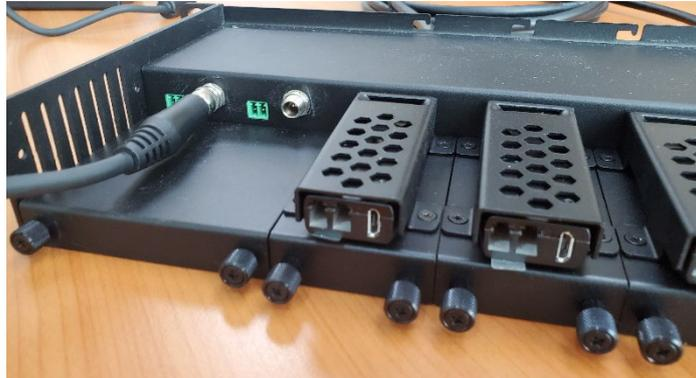
**Fig. 6: Mounting the Module bracket on BR-500.**
