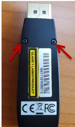
**Fig. 1: Remove two screws on the back side of the DisplayPort module**
